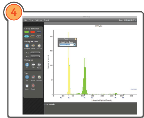
4. Tags with statistical information of the selected peak may be added and it is possible to select and view the selected objects. The whole process can also be done automatically.
