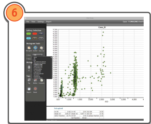
6. A scatter plot enables a plot with selected parameters. During setup it is possible to adjust for the optical features glare, dark current and diffraction.
